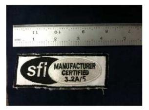
Example of a counterfeit label obtained by SFI (not attached to any suit). Note incorrect blue color, font, and wrong material:
